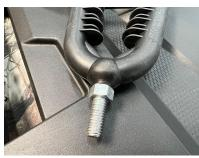
**Step 6:** Thread the Fork into the Anchor block. Screw the fork in as far as possible while stopping with it facing the desired direction. Then using a 9/16" Wrench tighten the nut snuggly against the Anchor which will secure it in place. Repeat for the other side.
